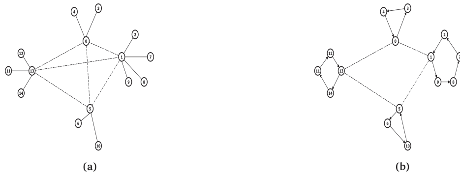
FIGURE 1. Basic and round-trip HLP networks. (a) A basic hub-and-spoke service network. (b) A typical round-trip hub-and-spoke service network.
