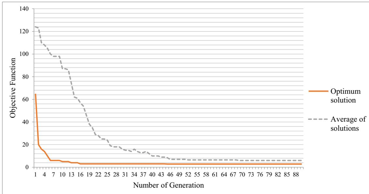
FIGURE 5. The convergence of NSGAI with tuned parameters.
